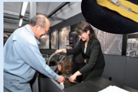
Clamping the elements in place using a pressing machine. The resulting fastener (insert)
