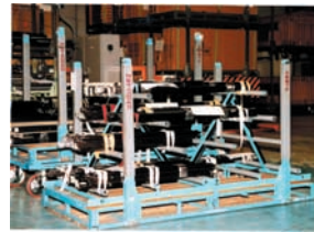
<Unpackaged delivery of each house unit> Sashes are placed on pallets for each building and delivered.
