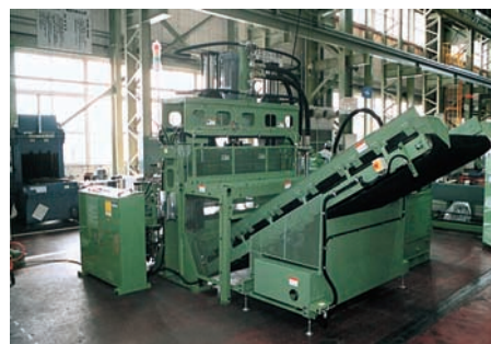
Aluminum formed material scrap disposal equipment
