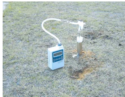
Collecting a soil gas sample
