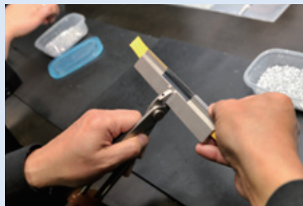
Clipping the tape into a jig and embedding the elements, setting them all in the same direction
