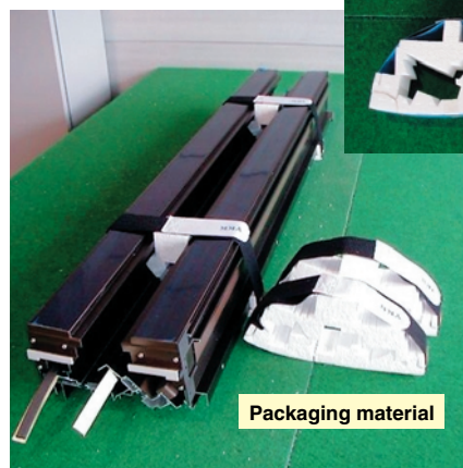
YKK has subsequently quit using all packaging materials. By using returnable packaging material of foam polyethylene and YKK surface fastener, we have realized zero packaging waste.
