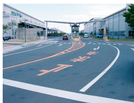
Front gate of Tohoku plant (YKK waste glass used as roadway subgrade)
