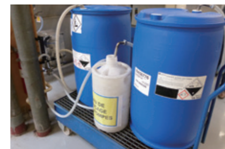
Automatic injection pump and solvent recovery device (YKK France S.A.R.L.)
