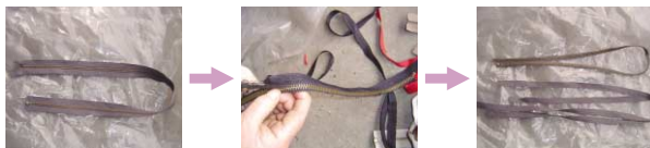
Metal and tape are separated and each material is recycled
