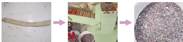
Injection fastener teeth (polyacetal), tape (polyester) are separated and reused
