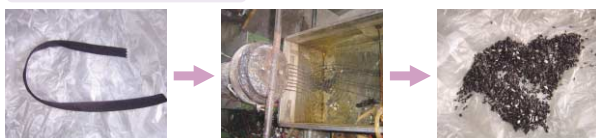
Resin fastener scraps are put through an extruder and reused as pellets
