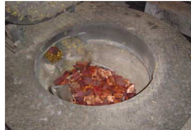
Round low-frequency melting furnace
