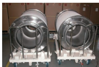
Improvement of bobbin transfer vehicles at the Dyeing Department (Portugal)
