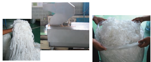
We installed a crusher to recycle imperfect tape scraps into cushion material for pillows, dolls, mats and other products (YKK Zipper Indonesia, PPD Plant)
