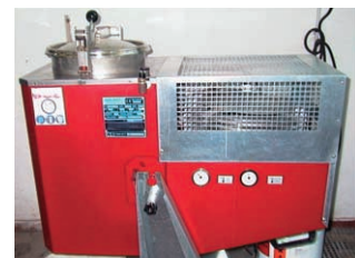
Used solvents are put into equipment for distillation and separation and the solvents are collected and reused (YKK Italia)
