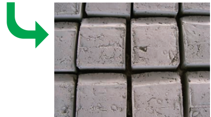
Cement and other materials are mixed with wastewater processing sludge to make blocks (YKK India)
